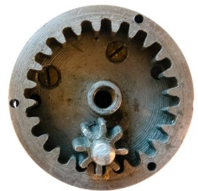
Figure 2: Bearing plate and shaft gear engaged with rotating ring gear.
